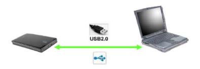
If the device installs with 2.5" SATA HDD and the PC/Laptop can provide enough current via USB, the device will be powered by USB interface, i.e. no external DC in power is needed in this mode.
